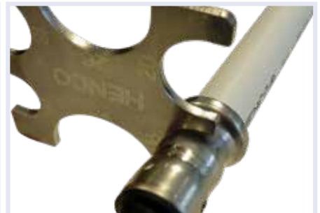
5. Rotate the tool 360° around the indented section and ensure that they mate perfectly together during this action as in step 4. Should this fail (for instance the distance is too great or there is an obstruction), then there is something wrong with the pressing in the connection. In this case we recommend that you make a completely new press connection and check the press machine using the jaws of the press tool.
