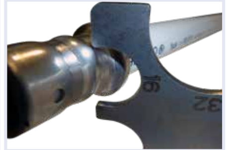
3. Place the corresponding cut-away section of the measurement tool on the indented section on the press sleeve.
