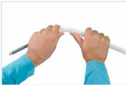
Bending with an internal bending spring
