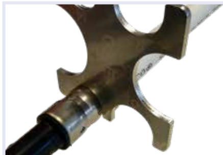
5. Rotate the tool 360° around the indented section and ensure that they mate perfectly together during this action as in step 4. Should this fail (for instance the distance is too great or there is an obstruction), then there is something wrong with the pressing in the connection. In this case we recommend that you make a completely new press connection and check the press machine using the jaws of the press tool.
