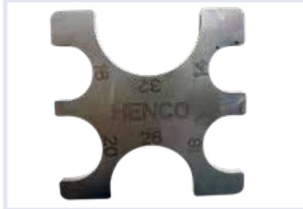
2. Find the corresponding \varnothing on the measurement tool.
