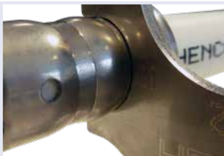
4. Note that the measurement tool and the indented section fit together perfectly.
